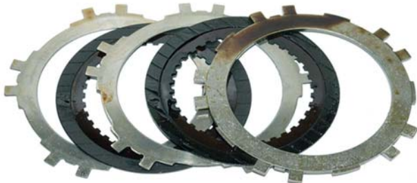
Automatic transmission clutch plates after cleanup with AMSOIL Engine and Transmission Flush reveal lighter glazing and varnish.
